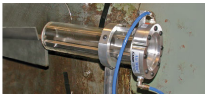
The Standard Air Wipe blows off the part and back into the centerless grinder.
